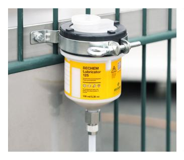
The lubricator is particularly suitable for supplying lubricant to difficult to access single lubrication points. It can be used at lubrication points of plain and roller bearings, linear guides, track rollers, shafts, seals, spindles, roller and toothed chains. The BECHEM Lubricator 125 provides perfect lubrication for up to one year and is proven by economy, time saving, working safety and hygiene.
