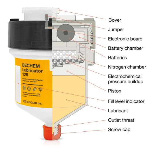
The BECHEM lubricator can be used independent of the position. After expiration of the operating time the lubricator will be replaced by a new unit.
